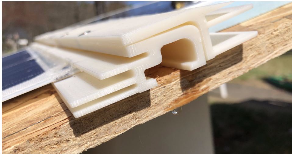
Figure 25: 2nd round of testing, leakage observed at the side at 18.4°
