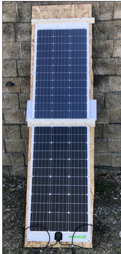
Figure 1: Full assembly of the prototype demonstrating the interface of two solar panels
