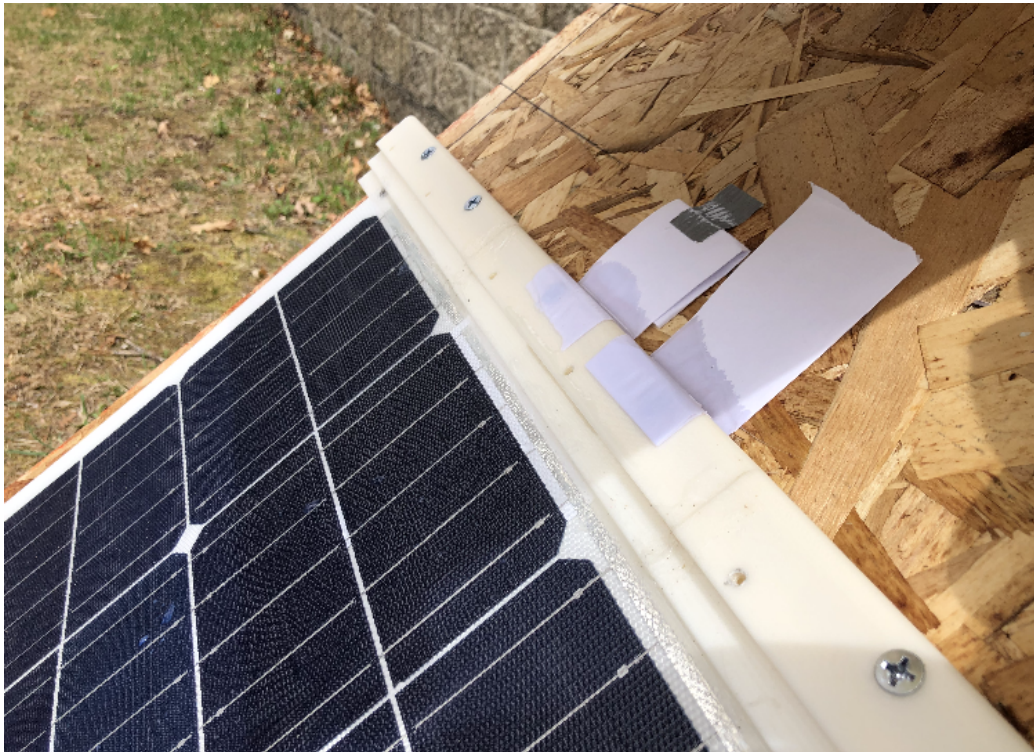
Figure 27: 3rd round of testing, 45° test with a removed fastener and paper on bottom rail
