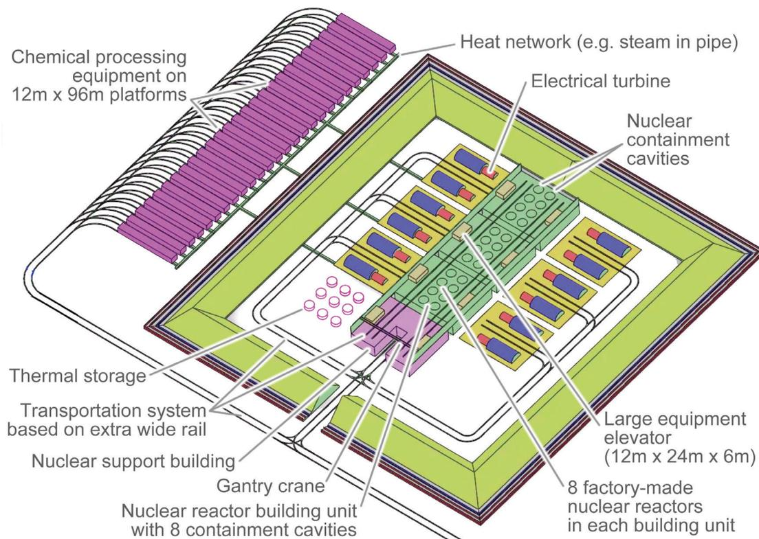
After regulators certify one facility, copies are made within a streamlined regulatory process. The equipment in the facility, including nuclear reactors, is mass produced in factories, to reduce cost.
