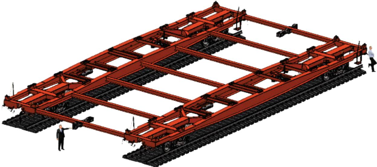
In this concept, railcars are sized at 12m by 24m and mount on double-tracks 12m apart. These railcars roll from factory, to dock near factory, to ship, to dock near power station, and then to power station.
