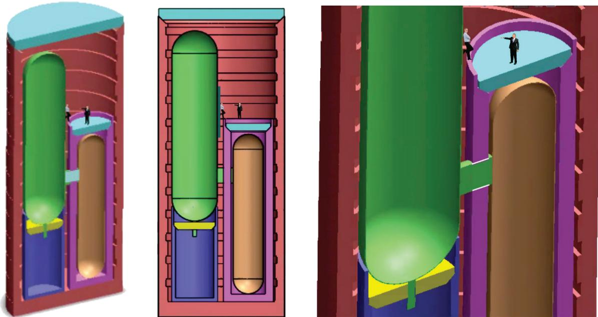
In some cases, reactor designers place one reactor into each containment cavity. However, in theory, one could place more than one into a cavity; or, spread out a large reactor among multiple cavities.
