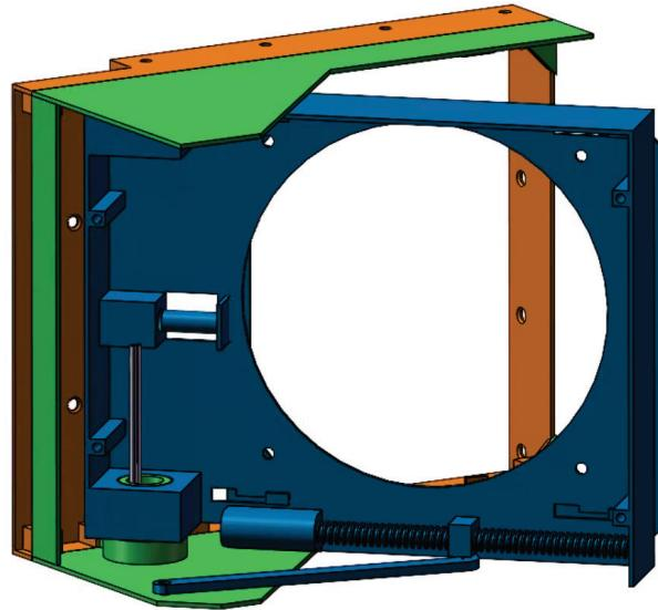
*Mechanism rotates pivot assembly (blue) 90 degrees and slides locking plate (on reverse side, not shown).*
