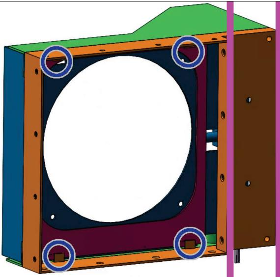
*Bracket (orange) secures to wood framing (violet) outside of duct. Fan vibration is transferred from fan to pivot assembly, to bracket, to wood wall framing (e.g. 2x4). Pivot assembly (blue) secures to bracket via sliding locking plate (burgundy) to reduce vibration.*
