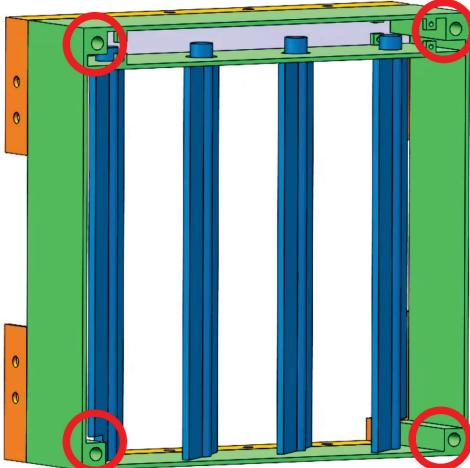
*Bracket (orange) is spot welded to duct and attaches to replaceable plug-in module (green) via 4 bolts (red).*
