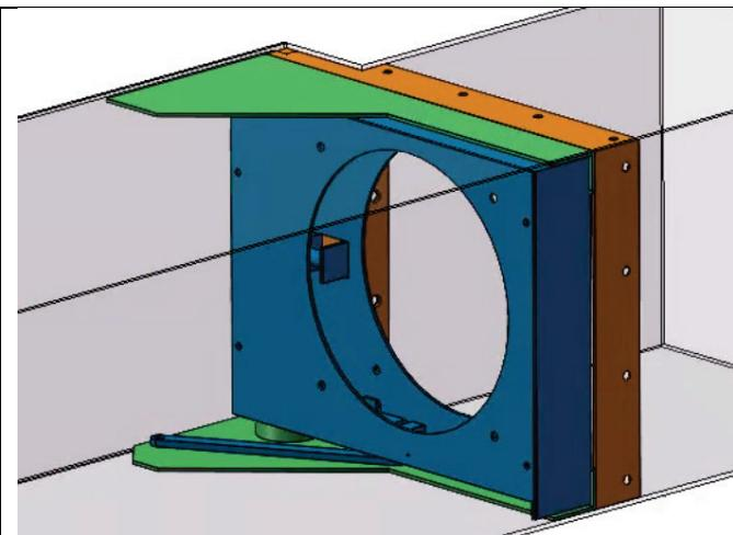
Bracket (orange) is spot welded to duct and attaches to module base (green) via 4 bolts. Circular fan (not shown) mounts within pivot assembly (blue). Replaceable module consists of base (green) and pivot assembly (blue). HVAC designer places this near vent, to allow access during replacement.
