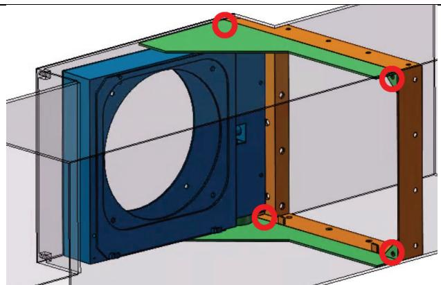
Module pivot assembly (blue) is shown here in storage bump-out position, possibly between wood wall framing (e.g. 2x4). During storage, only a small amount of central HVAC air is obstructed. Bolts (red) secure bracket to module base (green), supporting module replacement.
