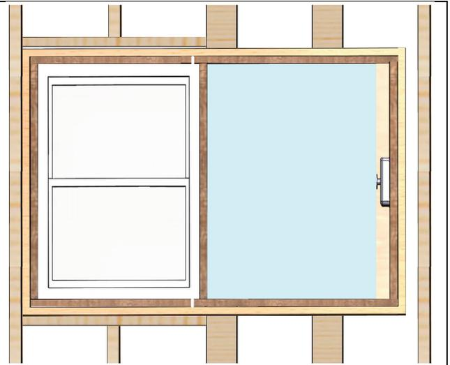
*Motor and worm-drive moves thermal cover (blue) into stow position behind drywall and out of view. Thermal cover assembly is pressed against drywall while insulation resides between thermal cover and exterior plywood sheathing. Moveable cover is light and therefore involves little force, ensuring safety. Internally, it contains Styrofoam like insulation several inches thick.*
