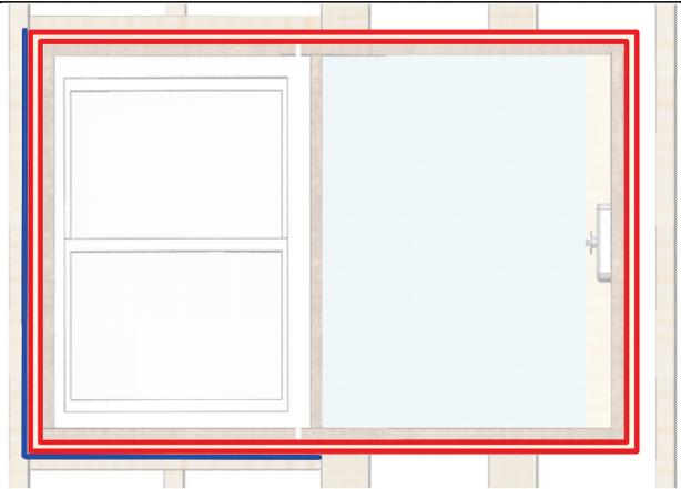
Thermal cover assembly outer frame (red) permanently attaches to wall framing (e.g. 2x6) along two surfaces (blue) via fasteners (e.g. screws) and/or glue bond. Everything inside assembly is the "thermal cover product" and is responsibility of thermal cover manufacturer; whereas everything outside is the responsibility of architect and carpenter. Wall framing is accurate to ~1cm whereas windows and window covers are significantly more precise due to internal seals.
