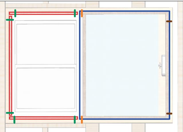
Replaceable plug-in module (blue) slides out after internal rails (red) are removed via bolts (green). Module (blue) is secured by bolts (orange) and pins (brown). Module contains components that will not last building lifetime. This includes moveable thermal cover, motor, worm-drive, electronics and gaskets. Standardization of module sizes ensures compatibility between different manufacturers; which increases access to replacement modules over building lifetime.
