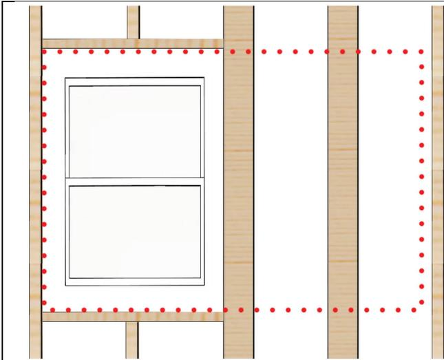
*Shown above is wood framing (e.g. 2x6) and window without thermal cover. Framing bears load and is not effected by thermal cover, with the possible exception of rotating several breams by 90 degrees. Window must transfer load from hurricane force winds to framing. Alternatively, thermal cover assembly bears no load, and therefore does not increase framing costs.*
