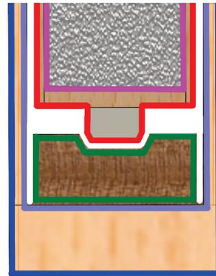
This is right side view of lower rail. Styrofoam-like insulation (violet) resides inside moveable cover (red). Thermal cover assembly (blue) and box inside assembly (purple) permanently attach to building. Plug-in module (green) houses cover and supports replacement. Carpenter seals permanent assembly (blue) to wall via caulk; and therefore prohibits airflow from inside wall to room.
