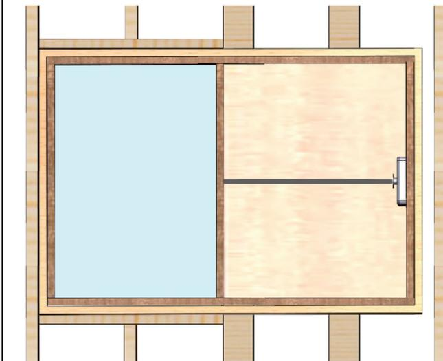
*Thermal cover (blue) seals airflow at perimeter via gaskets after being moved in front of window via mechanism. Shown here is worm drive, yet one could use alternative systems such as pulley/cable or linear gear.*
