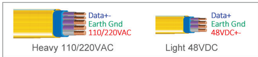
Figure 9.1: In theory, buildings could be supported by two power/data networks, one for large loads, and one for small.
