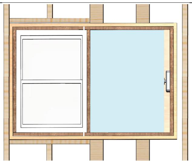
*Motor and worm-drive moves thermal cover (blue) into stow position behind drywall and out of view. Thermal cover assembly is pressed against drywall while insulation resides between thermal cover and exterior plywood sheathing. Moveable cover is light and therefore involves little force, ensuring safety. Internally, it contains Styrofoam like insulation several inches thick.*
