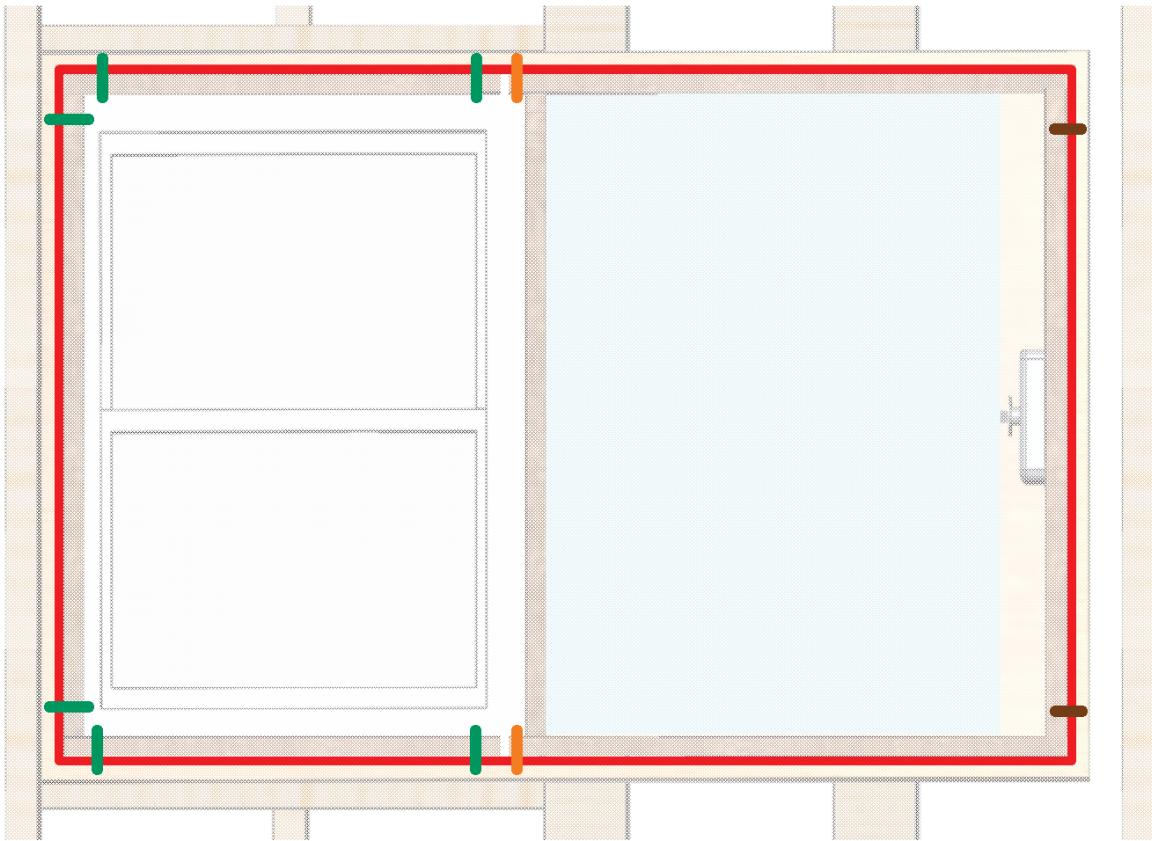
This means any product that meets these requirements will plug-and-play into an existing frame. Replacement gear consist of one plug-in module and three removable rails. Subsequently, manufacturers control: entire contents of module, gaskets, mechanics, motor, electronics, and different thermal designs.
