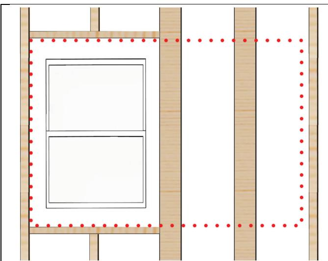
*Shown above is wood framing (e.g. 2x6) and window without thermal cover. Framing bears load and is not effected by thermal cover, with the possible exception of rotating several breams by 90 degrees. Window must transfer load from hurricane force winds to framing. Alternatively, thermal cover assembly bears no load, and therefore does not increase framing costs.*
