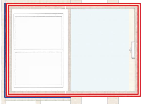
Thermal cover assembly outer frame (red) permanently attaches to wall framing (e.g. 2x6) along two surfaces (blue) via fasteners (e.g. screws) and/or glue bond. Everything inside assembly is the "thermal cover product" and is responsibility of thermal cover manufacturer; whereas everything outside is the responsibility of architect and carpenter. Wall framing is accurate to ~1cm whereas windows and window covers are significantly more precise due to internal seals.
