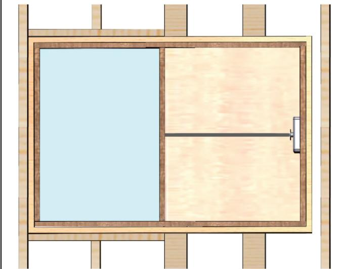
*Thermal cover (blue) seals airflow at perimeter via gaskets after being moved in front of window via mechanism. Shown here is worm drive, yet one could use alternative systems such as pulley/cable or linear gear.*
